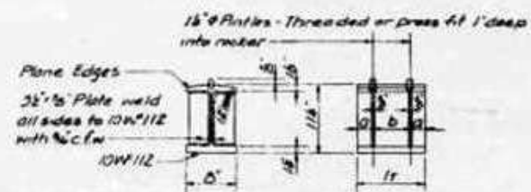
DETAIL OF FIXED BEARING
