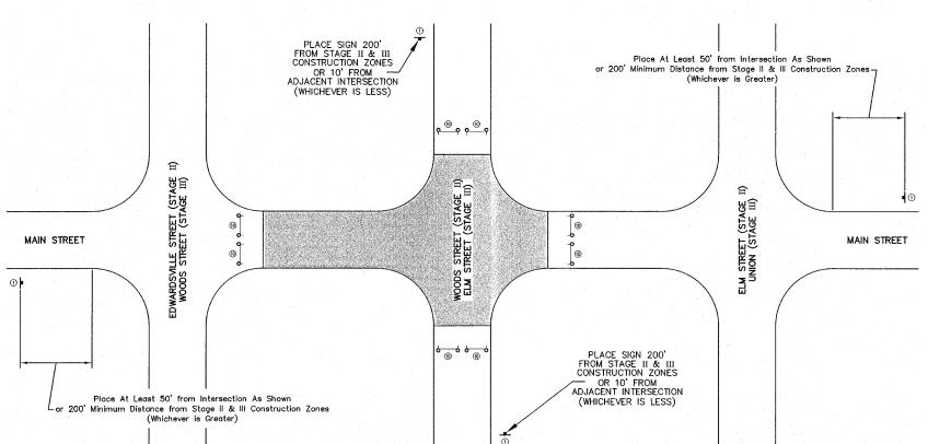
CONSTRUCTION ZONES II & III (CLOSED TO VEHICULAR TRAFFIC) → TYPE III BARRICADE WITH FLASHING LIGHTS
