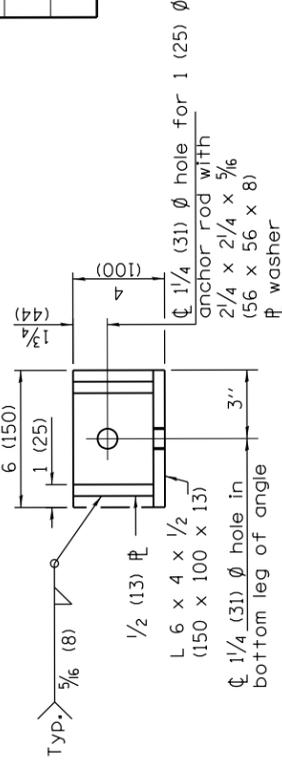
**REINFORCEMENT ANGLE DETAIL**
