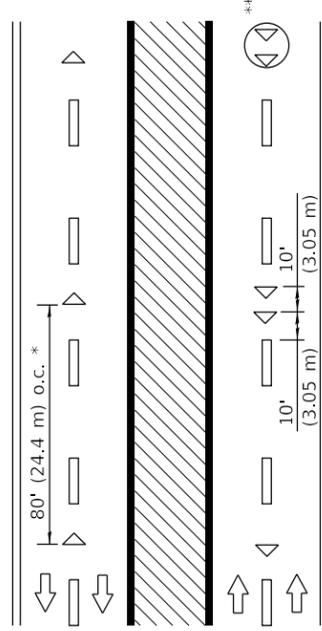
\* Reduce to 40' (12.2 m) o.c. on curves where advisory speeds are 10 mph (15 km/h) lower than posted speeds.
