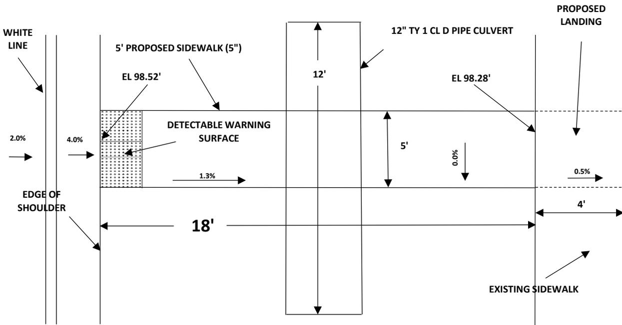
\* ALL ELEVATIONS ARE RELATIVE TO TEMPORARY BENCHMARK SET IN CONCRETE STA 5+25, 88' RT (EL 100.00)
