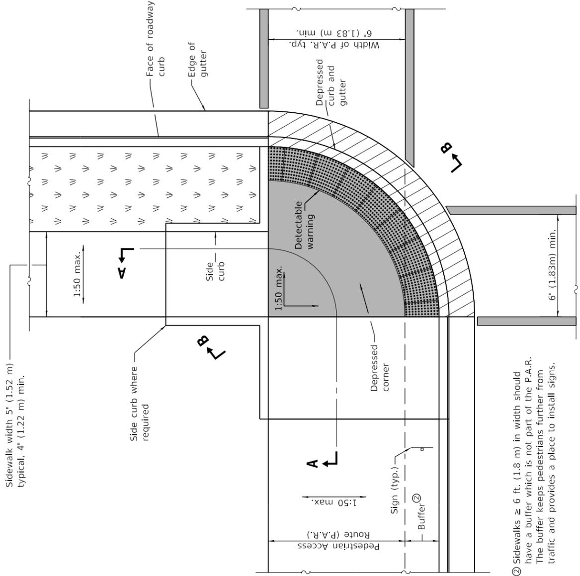
② Sidewalks  $\geq$  6 ft. (1.8 m) in width should have a buffer which is not part of the P.A.R. The buffer keeps pedestrians further from traffic and provides a place to install signs.
