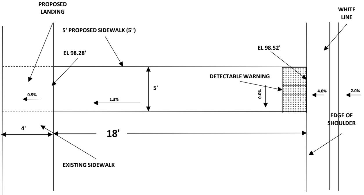
\* ALL ELEVATIONS ARE RELATIVE TO TEMPORARY BENCHMARK SET IN CONCRETE PAD STA 5+25, 88' RT (EL 100.00)
