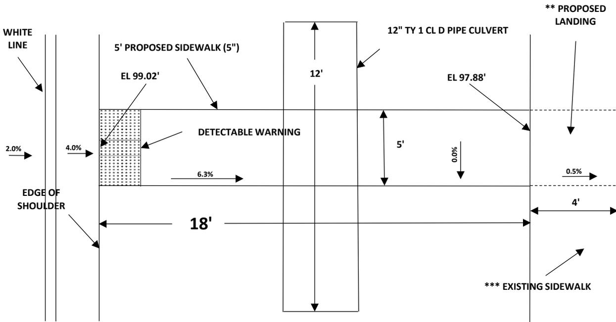
\* ALL ELEVATIONS ARE RELATIVE TO TEMPORARY BENCHMARK SET IN SE CONCRETE PAD STA 5+25, 88' RT (EL 100.00)
