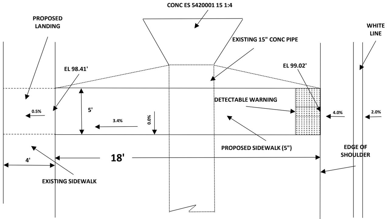
\* ALL ELEVATIONS ARE RELATIVE TO TEMPORARY BENCHMARK SET IN CONCRETE PAD STA 5+25, 88' RT (EL 100.00)
