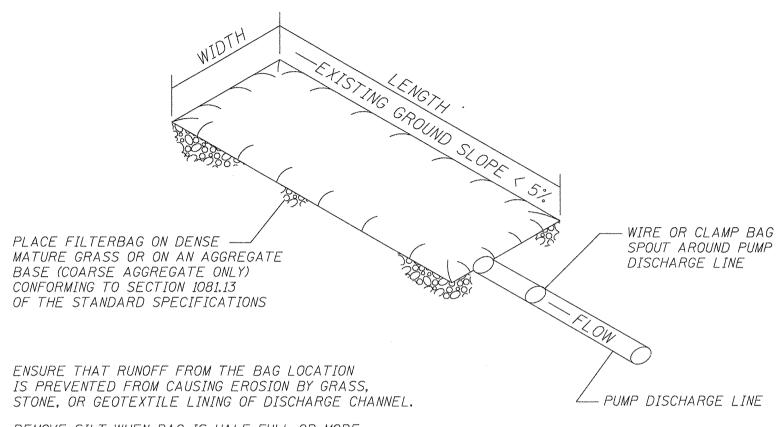
REMOVE SILT WHEN BAG IS HALF FULL OR MORE OFTEN IF RECOMMENDED BY THE MANUFACTURER. DISPOSE OF SILT BY TRANSPORTING THE FILLED BAG TO DISPOSAL AREA. SLIT THE BAG, BLEND SILT INTO EXISTING TOPOGRAGHY, SEED AND MULCH
