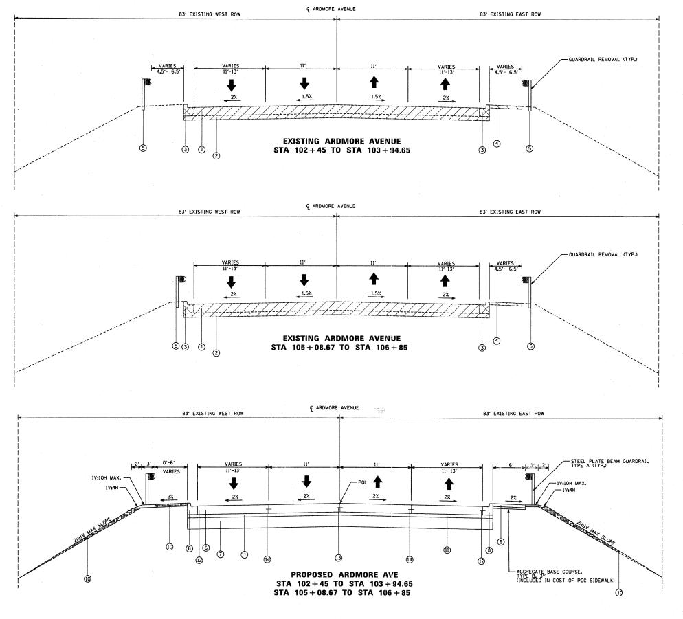
EXIST. PORTLAND CEMENT CONCRETE PAVEMENT, 8" (JOINTED)
