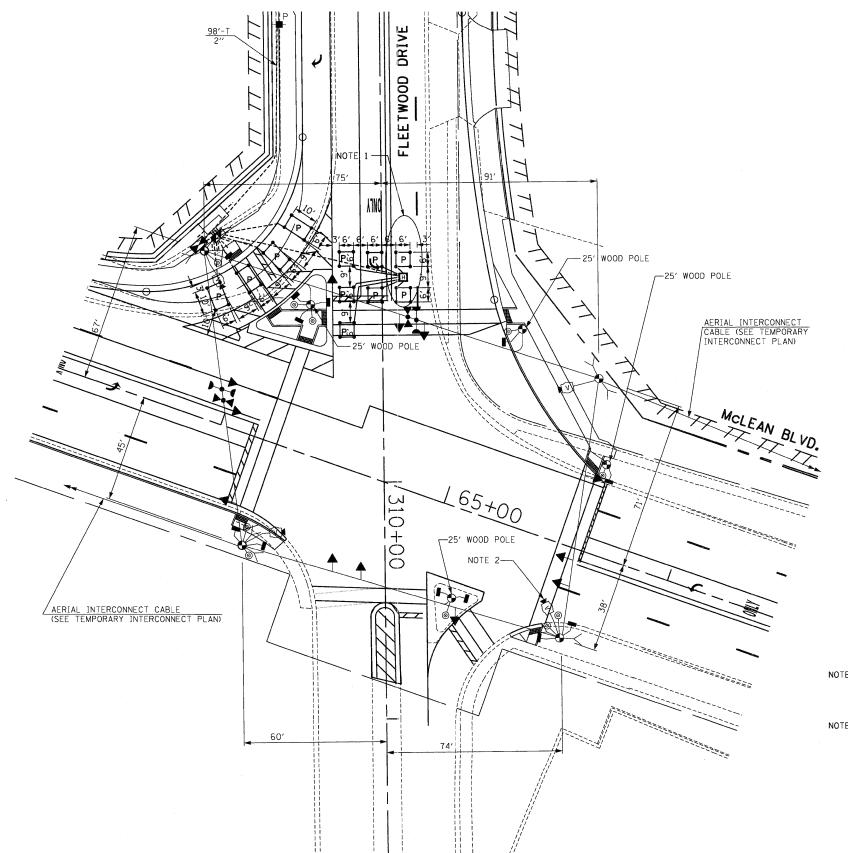
NOTE 1: THE DETECTOR LOOPS IN THE WESTBOUND LANE SHALL BE DISABLED UNTIL THE PERMANENT SIGNAL INSTALLATION IS PUT IN OPERATION. THE DETECTOR LOOP CABLES SHALL BE CONNECTED INTO THE TEMPORARY CONTROLLER.
