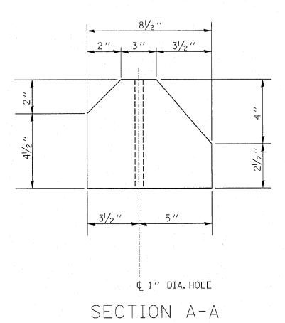
EX & PR BUMPER BLOCKS TO BE FASTENED TO PR BIT. SURF. W/ 3/4" Ø x 24" STEEL SPIKES W/ CAPS APPROVED BY THE ENGINEER
