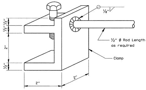
Notes: Pop rivet the  $\frac{1}{8}$ " x 1" bar to drain extension. Weld or securely attach rod to both the clamp and bar stiffener. Use 3/6" stainless steel pop rivets of sufficient length.
