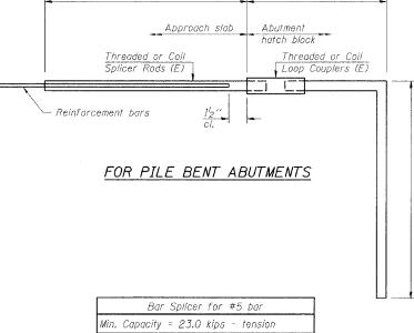
Min. Pull-out Strength = 9.2 kips - tension No. Required = N/A
