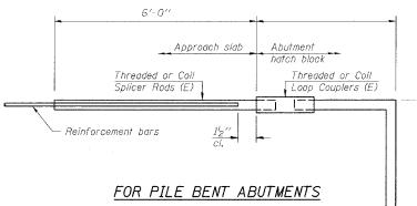
Bar Splicer for #5 bar Min. Capacity = 23.0 kips - tension Min. Pull-out Strength = 9.2 kips - tension o. Required = N/A
