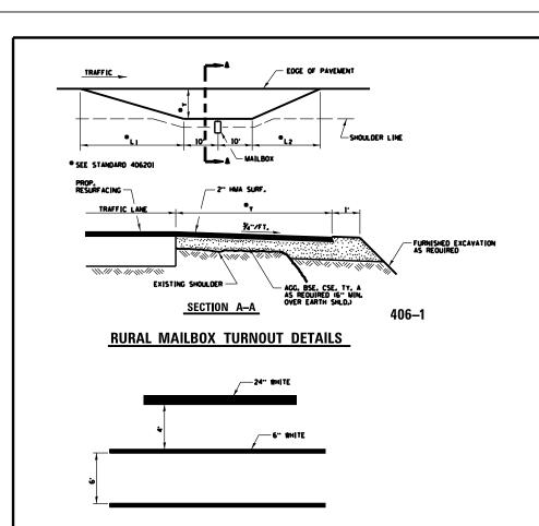
TYPICAL SPACING DETAIL FOR CROSSWALKS AND STOP BARS
