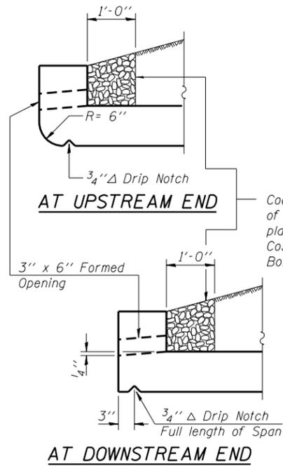
Coarse aggregate full length of both headwalls. To be placed by Grading Contractor. Cast included with Concrete Box Culverts.
