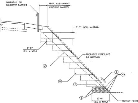
TYPICAL BENCHING DETAIL FOR EMBANKMENT
