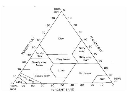
The mechanical analysis should show that the % sand, % silt, and the % clay must yield a silt loam soil. See the attached Textural Classes diagram above. To determine the class plot a line parallel to the % clay axis starting the line at the value of the % silt. Plot another line parallel to the % sand axis starting the line at the value of the % clay. The intersection of these lines should be in the silt loam region, for the soil to be approved.
