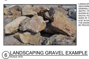
LANDSCAPING GRAVEL SHALL BE WEATHERED LIMESTONE AND GENERALLY MATCH THE COLORS (BUFFS, TANS, GRAY) AND SHAPE SHOWN IN THE PICTURE, REFER TO DIGITAL PDF FOR COLORS. THE SIZES OF THE STONES SHALL BE 8-36" IN DIAMETER, AS APPROVED BY THE ENGINEER. COLOR IMAGE WILL BE PROVIDED UPON REQUEST.
