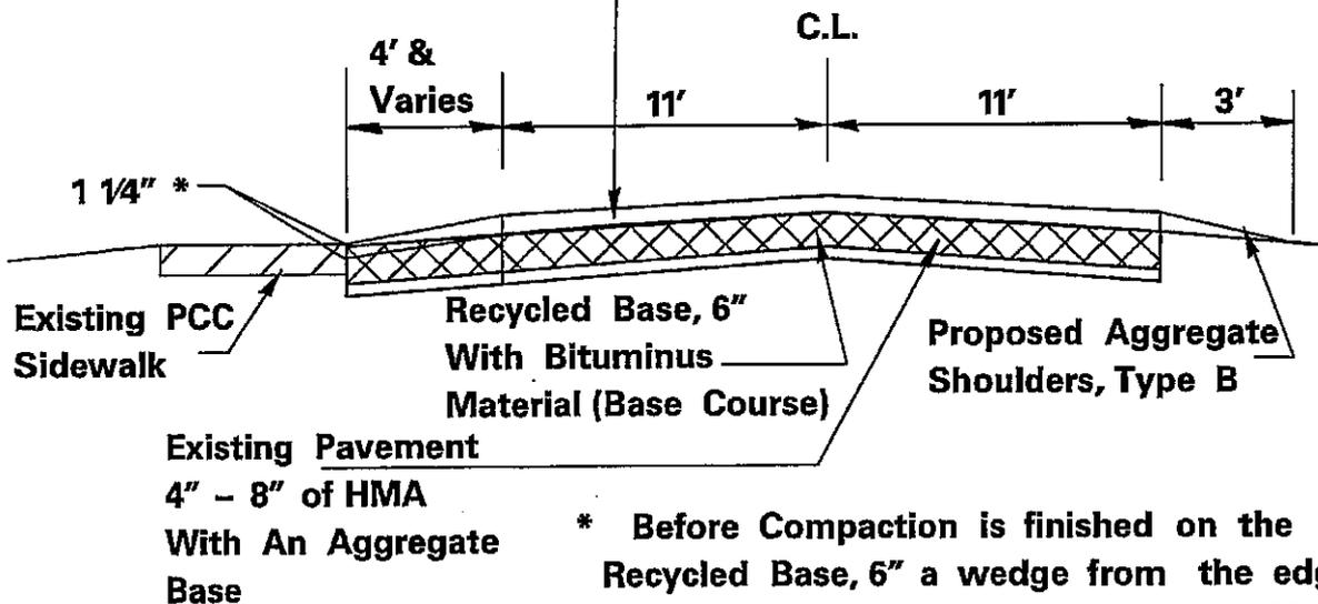
\* Before Compaction is finished on the Recycled Base, 6" a wedge from the edge of shoulder down to 1 1/4" at sidewalk will be needed to allow for the HMA Surface Course.
