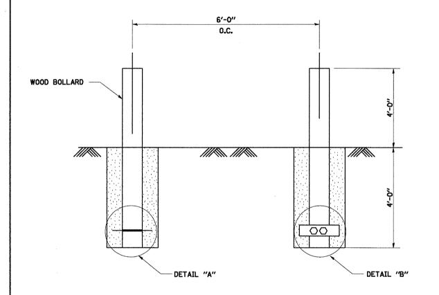
TOPS OF BOLLARDS SHALL BE SLOPED SO WATER DOES NOT PUDDLE
