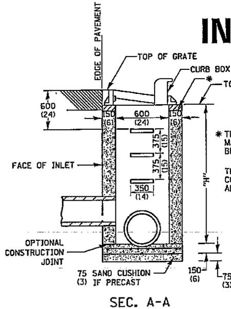
\* THE WALL ADJUSTMENTS SHALL BE MADE WITH CONCRETE BUILDING BRICK OR CLASS SI CONCRETE.
