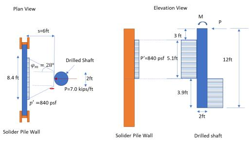
Exhibit 3: Additional Pressure from Drilled Shafts onto the Solider Pile Wall
