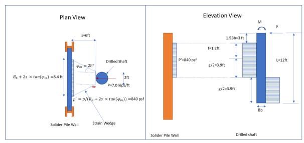
This exhibit shows the most critical condition. When the load on top of the drilled shafts changes directions, the additional pressure will act to a deeper depth on the wall, which is less critical than the condition shown above.
