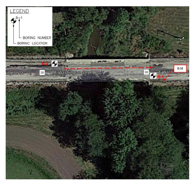
B.M. – BENCHMARK IS LARGE NAIL WITH RIBBON IN GROUND. STATIONING RUNS EAST STARTING AT CENTER WEST EDGE OF BRIDGE.
