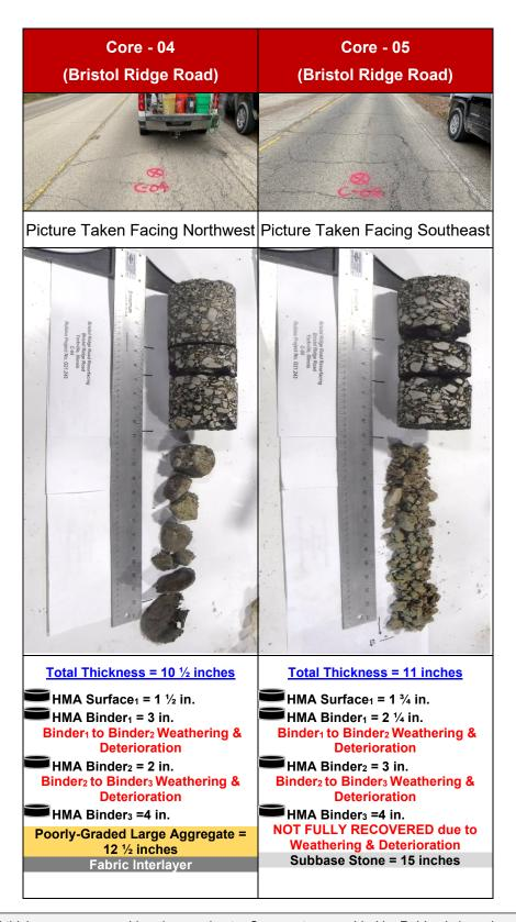
The referenced thicknesses are considered approximate. Commentary provided by Rubino is based on our observation in the laboratory; **Crack** = vertical through cross section; **Weathering** = rounded edges & degradation of asphalt and **Deterioration** = horizontal crack. Pavement and subbase type and thickness may vary between core locations. Any comments on the condition of the material are considered our opinion and should be verified by the design engineer.
