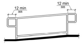
Method of Measurement: The handrail quantity will be measured along the top rail per FOOT.
