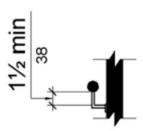
Circular Cross Section. Handrail gripping surfaces with a circular cross section shall have an outside diameter of 1½ inches minimum and 2 inches maximum.
