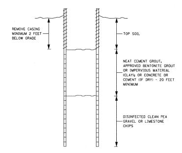
NOTE: ABANDONED DUG AND BORED WELLS CAN ALSO BE SEALED WITH ALTERNATING LAYERS OF APPROVED BENTONITE GROUT AND AGRICULTURAL LIME (LIMESTONE FINES) OR COMPLETELY FILLING WITH CONCRETE, CEMENT GROUT, OR IMPERVIOUS MATERIAL SUCH AS CLAY.
