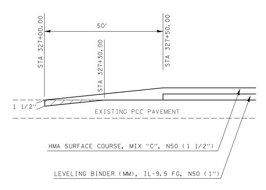
PCC SURFACE REMOVAL, BUTT JOINT
