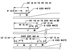
FULL SIZE LETTERS 8' (2.4 m) AND ARROWS SHALL BE USED.  $\P$  AREA = 15.6 SO. FT. (1.5 m<sup>2</sup> )  $\parallel \parallel \parallel$  AREA = 20.8 SO. FT. (1.9 m<sup>2</sup>)
