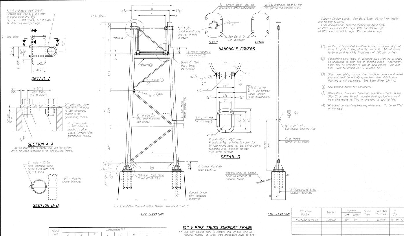
support frame. If used, weld procedure must be preapproved by Engineer and joint shall receive 100% RT or UT (tension criteria) at Contractor's expense.
