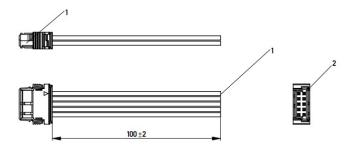
18AWG WIRE ARE TO BE PARTIALLY STRIP 10MM FROM END
