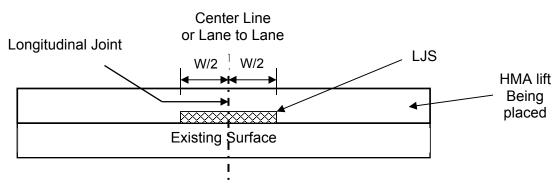
The width and minimum application rate shall be according to the following table:
