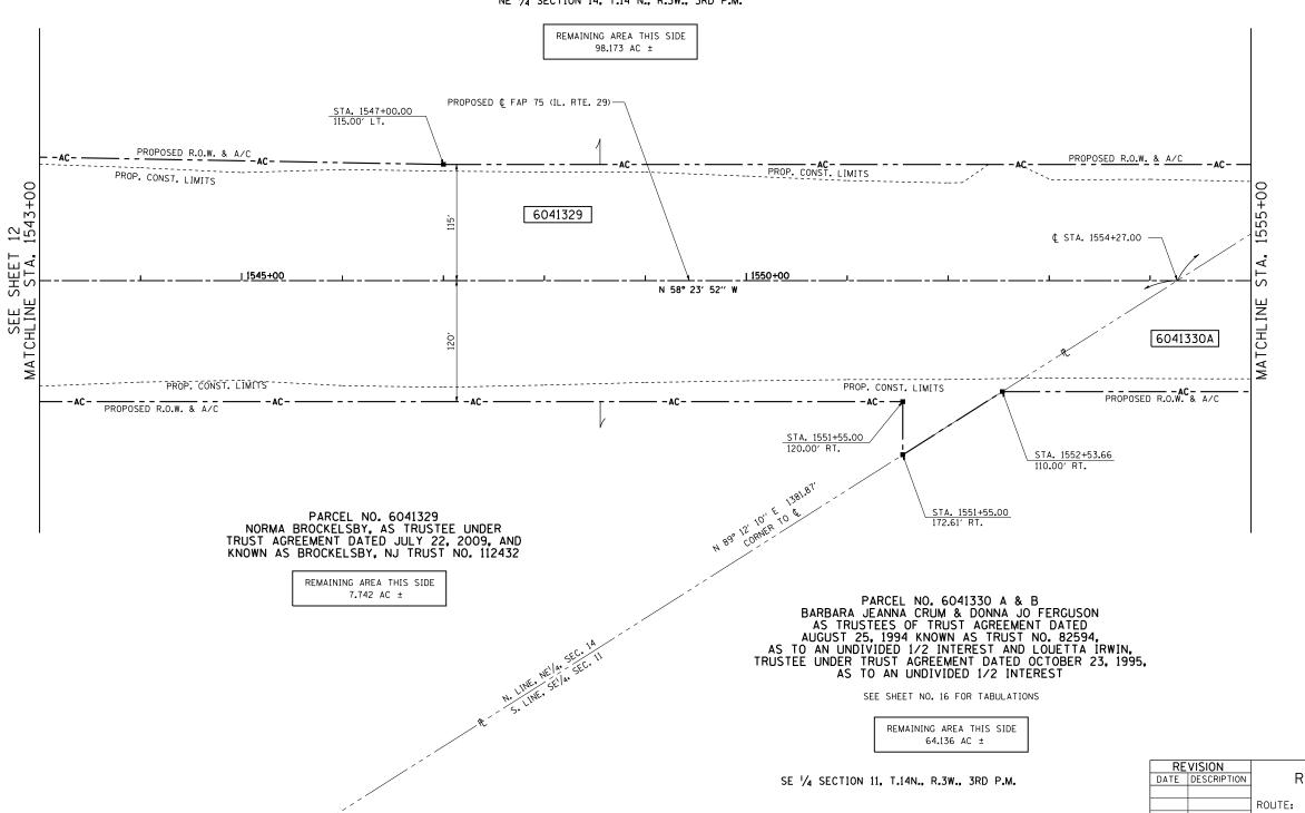
1" IRON PIPE OVER STONE (FOUND) SE CORNER, SECTION 11 T14N, R3W, 3RD P.M. STA. 1452+60.24, 740.44' RT.
