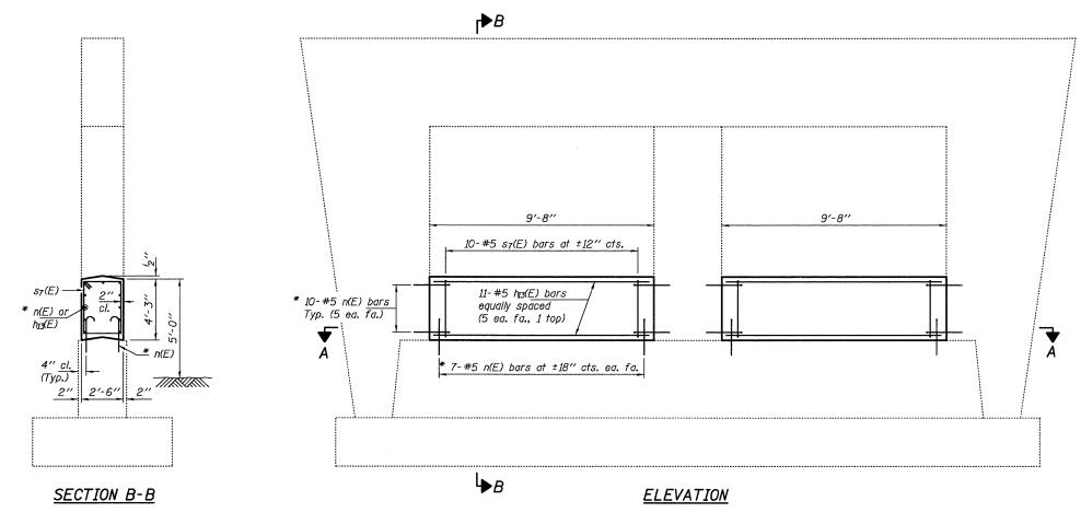
\* Epoxy grout n(E) bars in 9" min. holes according to Article 584 of the Standard Specifications.
