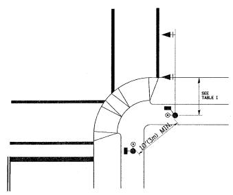
RECOMMENDED PUSHBUTTON LOCATIONS FOR ACCESSIBLE PEDESTRIAN SIGNALS SHALL BE IN ACCORDANCE WITH THE CURRENT MUTCO (SEE NOTE 1). TO MEET MUTCO REQUIREMENTS, PEDESTRIAN SIGNAL PUSHBUTTONS MAY HAVE TO BE MOUNTED ON A SEPARATE POST.
