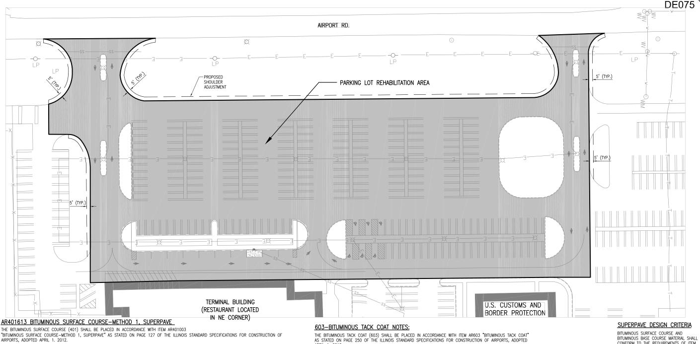
THIS ITEM OF WORK SHALL CONSIST OF CONSTRUCTING: A 2 INCH SURFACE LIFT OF BITUMINOUS SURFACE COURSE-METHOD 1, SUPERPAVE ON THE EXISTING BITUMINOUS BASE.
