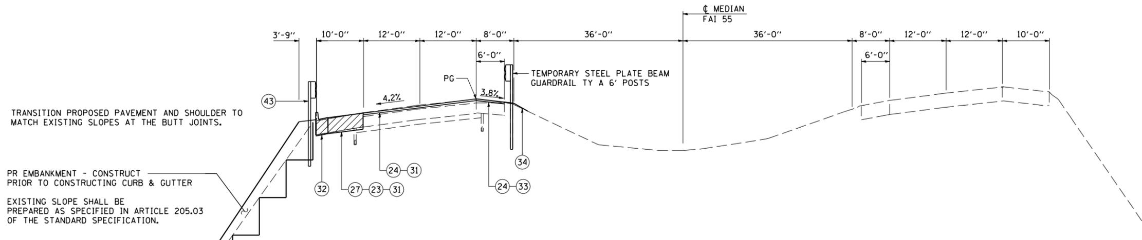
RECONSTRUCT SB OUTSIDE SHOULDER WITH HMA BASE COURSE 10 3/4" AND HMA SURFACE COURSE, MIX "E", N105 1/2" AT THE FOLLOWING LOCATIONS
