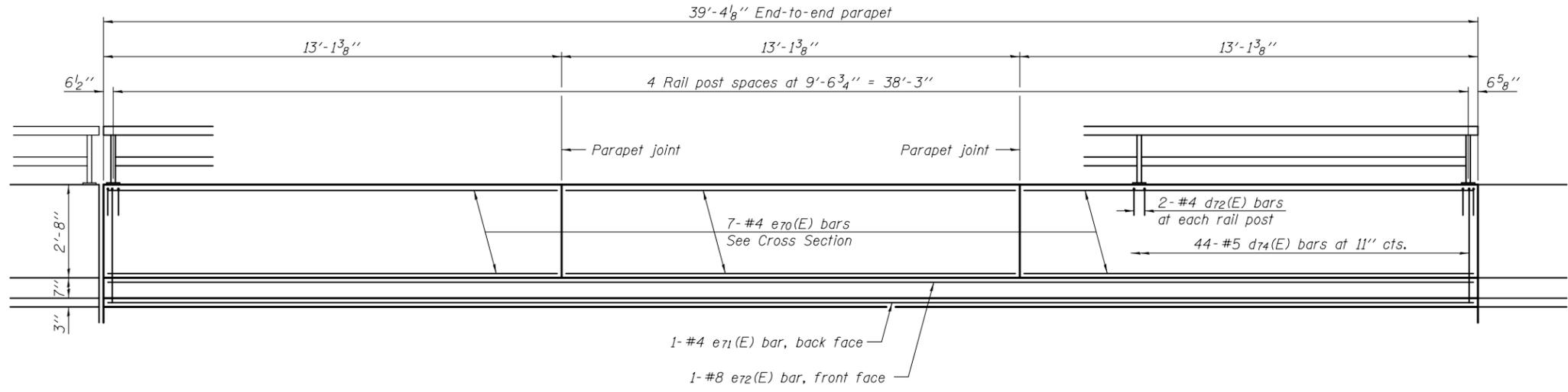
**INSIDE ELEVATION OF WEST ROADWAY PARAPET**
