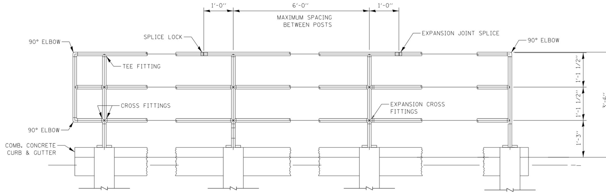
**TYPICAL HANDRAIL POST ELEVATIONS**
