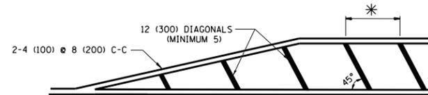
\* FOR MEDIAN LENGTHS WHERE DIAGONAL SPACING CANNOT BE ATTAINED, USE 5 (FIVE) EQUALLY SPACED DIAGONAL LINES.
