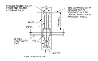
UNDERDRAIN COLLECTION STRUCTURE (CS) DETAIL NOT TO SCALE
