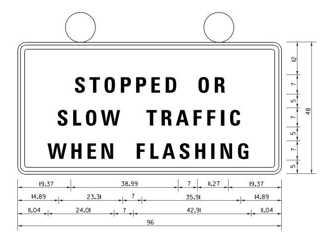
Stopped Or Slow Traffic When Flashing; 2.25" Radius, 1.00" Border, 0.63" Indent, Black on Orange; "STOPPED OR" D 2K; "SLOW TRAFFIC" D 2K; "WHEN FLASHING" D 2K;
