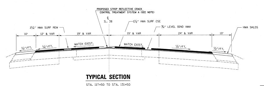
NOTE: STRIP REFLECTIVE CRACK CONTROL TO BE PLACED ALONG CENTERLINE OR OTHER WIDENING CRACKS AS DIRECTED BY THE ENGINEER.
