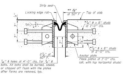
The strip seal shall be made continuous and shall have a minimum thickness of  $\frac{1}{4}$ ". The configuration of the strip seal shall match the configuration of the Locking Edge Rails. Open or "webbed" strip seal gland configurations are not permitted. The gland shall be sized for a maximum rated movement of 4 inches.
