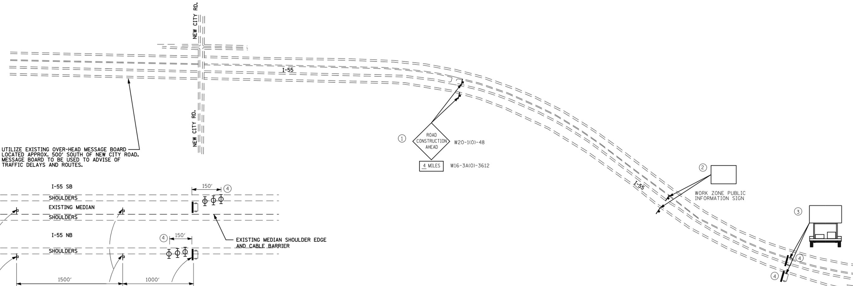
UTILIZE EXISTING OVER-HEAD MESSAGE BOARD LOCATED APPROX. 500' SOUTH OF NEW CITY ROAD. MESSAGE BOARD TO BE USED TO ADVISE OF TRAFFIC DELAYS AND ROUTES.
