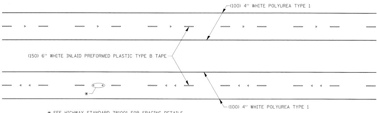
\* SEE HIGHWAY STANDARD 781001 FOR SPACING DETAILS. USE DOUBLE MARKERS WHEN ADT  $\geq$  25,000.
