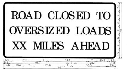
Permit Loads - Loads Over 13 Feet; 3.0" Radius, 1.3" Border, Black on Orange; [ROAD CLOSED TO] D; [OVERSIZED LOADS] D; [XX MILES AHEAD] D;
