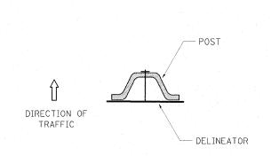
DELINEATORS SHALL BE INSTALLED ACCORDING TO STANDARD 635001 EXCEPT THAT THE POST SHALL BE ROTATED 180°. THE POST WILL HAVE THE WIDE SIDE FACING TRAFFIC AND THE DELINEATOR ATTACHECD AS SHOWN ABOVE.
