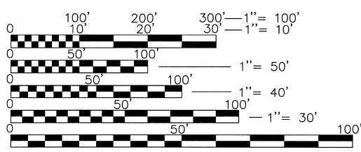
FULL SIZE PLANS HAVE BEEN PREPARED USING STANDARD ENGINEERING SCALES. REDUCED SIZED PLANS MAY NOT CONFORM TO STANDARD SCALES. IN MAKING MEASUREMENTS ON REDUCED PLANS, THE ABOVE SCALES MAY BE USED.
