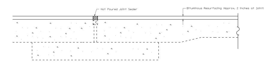
NOTE: CONTRACTOR TO SURFACE OVER EXISTING PREFORMED JOINT SEALER. UPON COMPLETION OF RESURFACING, CONTRACTOR IS TO SAW CUT AT THE EDGE OF THE PJS AND REMOVE THE BITUMINOUS MATERIAL, COST TO BE INCLUDED WITH BITUMINOUS RESURFACING ITEMS.
