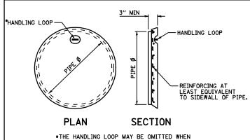
\*THE HANDLING LOOP MAY BE OMITTED WHEN THE CAP IS PLACED IN A BURIED INSTALLATION.
