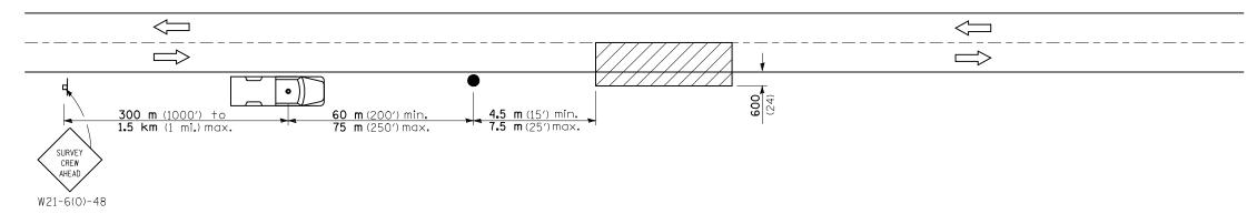
FLAGGER SHALL BE EQUIPPED WITH AND REQUIRED TO USE A HIGH INTENSITY, OR HIGH PERFORMANCE " STOP - SLOW "
