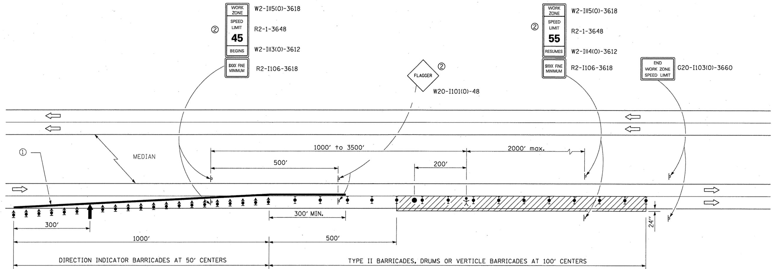
SEE TRAFFIC CONTROL AND PROTECTION STANDARD 701400 (SPECIAL) FOR APPROACH TO LANE CLOSURE DETAILS
