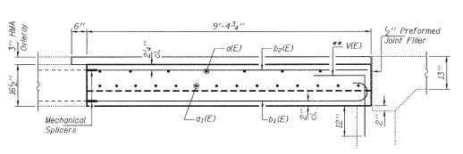
SECTION THRU THICKENED EDGE OF SLAB Dims. at Rt. L
