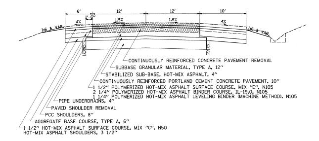
NOTE: EXISTING UNDERDRAINS AT SHADY OAKS 30" DEEP TO BE REMOVED AND INCLUDED IN THE COST OF EXCAVATION.
